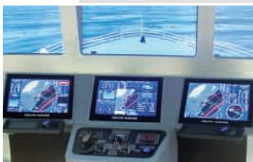
Kelvin Hughes Integrated Bridge System Screen format 16:10
